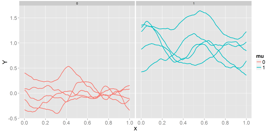
Figure 2.1: The outcomes of two Gaussian processes with the same covariance function and different constant means.
