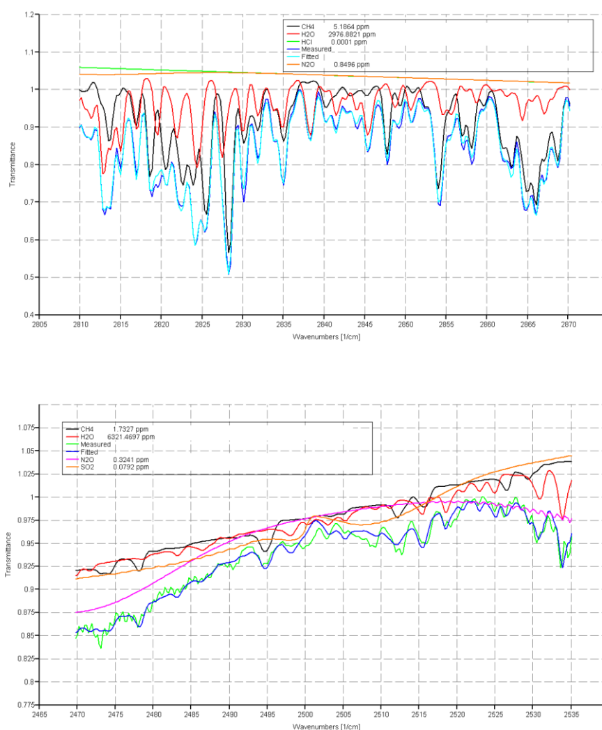
Figure 25. Spectral fitting of solar-FTIR measurements at Nyiragongo. The upper plot shows the case for HCl, along with the interfering species CH 4 , H 2 O and N 2 O. The lower plot shows the fitting for SO 2 , in the region where also CH 4 , H 2 O and N 2 O absorb. The SO 2 /HCl molar ratio out of 37 measurements was in the range 24.3 \pm 1.8 (Nov. 2013) and from 826 spectra the molar ratio was 18 \pm 1.5 (Mar. 2014)
